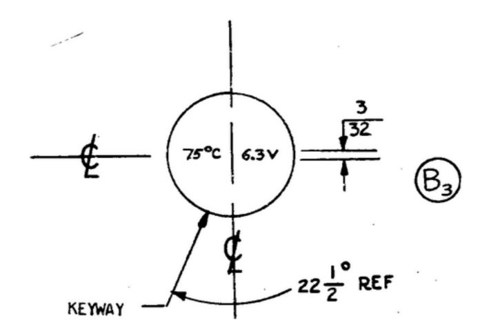
LETTERING TO BE PLACED WITH REF TO KEYWAY ON SOCKET
